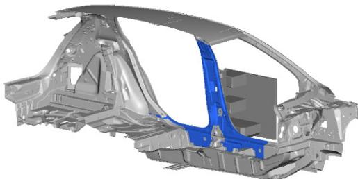
Manufacturers need as much insight into the design as possible. And one key area where typical crash simulations fail is in modeling how metal is going to tear or fracture. Since a metal fracture dramatically changes a vehicle’s structural integrity, predicting where and how these tears will happen is absolutely critical in the design process.
