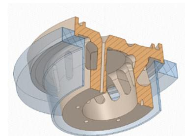
**ACTIVE NOZZLES:** Using CFD, Tetra Pak developed the active nozzle. The nozzle allows gas to flow and sterilize every part of the machine as well as the aseptic chamber. The process assures effective package sterilization.
