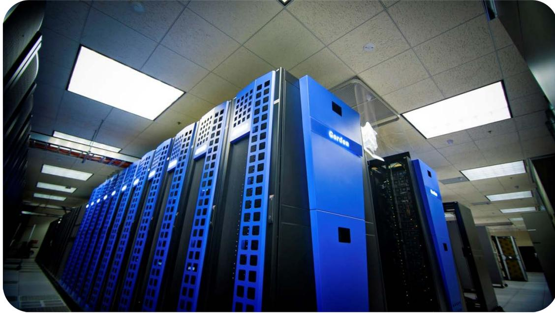
**Figure 2:** Gordon consists of 21 racks in a compact, energy-efficient 48U form factor
