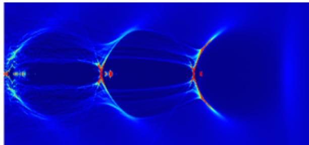
An image captured from the computer simulation of the plasma wakefield as it evolves over the length of the nine-centimeter channel.
